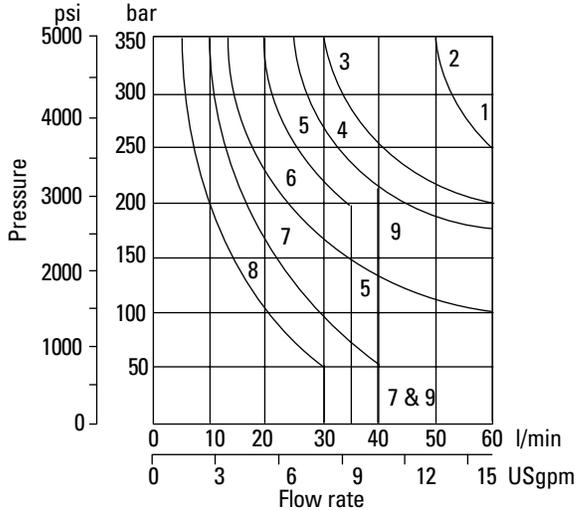
**Graph 5** AC solenoid valves with dual-frequency coils operating at 60 Hz
