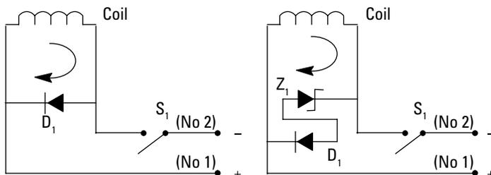
NOTE: These surge suppression devices are "Polarity Dependent." Proper biasing conditions must be met when installing/connecting a coil in a system.
