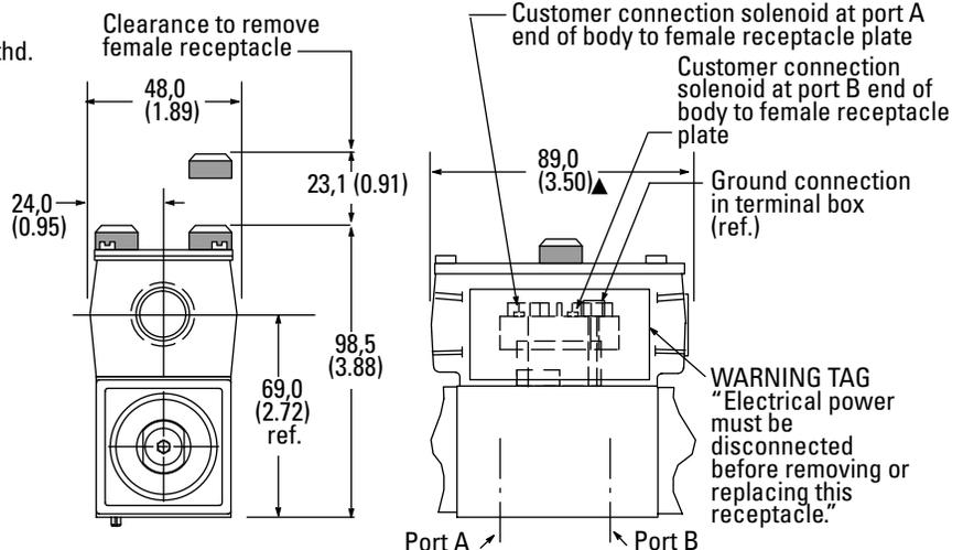
▲ The conduit box dimensions used for the PA/PBW type connector are different from those on the other "F" type coil models.
