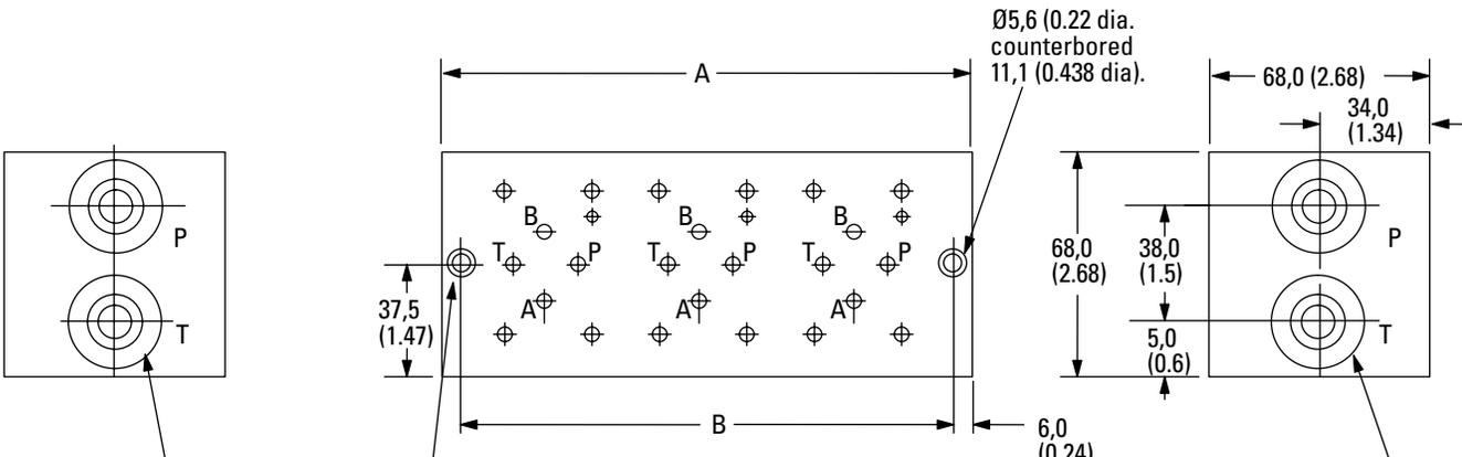
These two ports are present in 4, 5, and 6 station models. Optional in 2 and 3 station models, specify DGMS-3-2EX-1\*-\* or DGMS-3-3EX-1\*-\*
